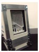
9. Ensure the power trip switch is switched on, then plug the flightcase to the mains electric. Fans should come on and the pop up will start to inflate. After 2 to 3 minutes the pop up should be inflated and holding its structure and buoyancy.
