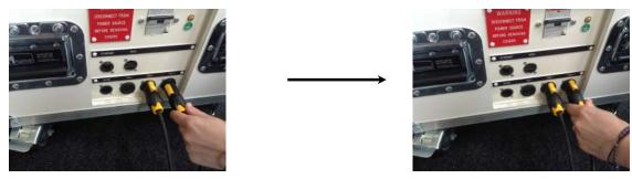
**Top Tip!**Cables should go in and twist to connect. You should hear a click.
