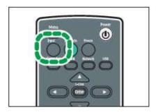
3. The input signal is detected automatically and the image is projected. The input signal changes each time the [Input] button is pressed.
