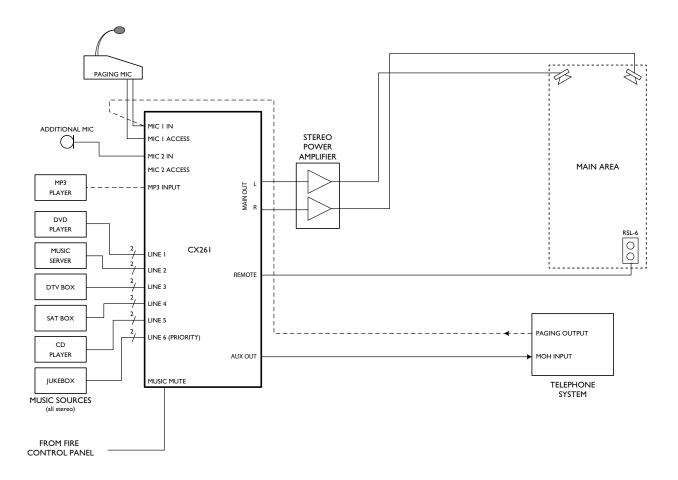
The example shows a CX261 used to provide stereo music, announcements and paging in a multi-purpose area. The area can set its own music source and volume by means of the local RSL-6 remote control plate (optional). Music source and level could be set from the front panel of the mixer itself if preferred.
